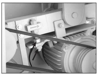
Figure 48. Motor mount nuts (1 of 2 shown).
